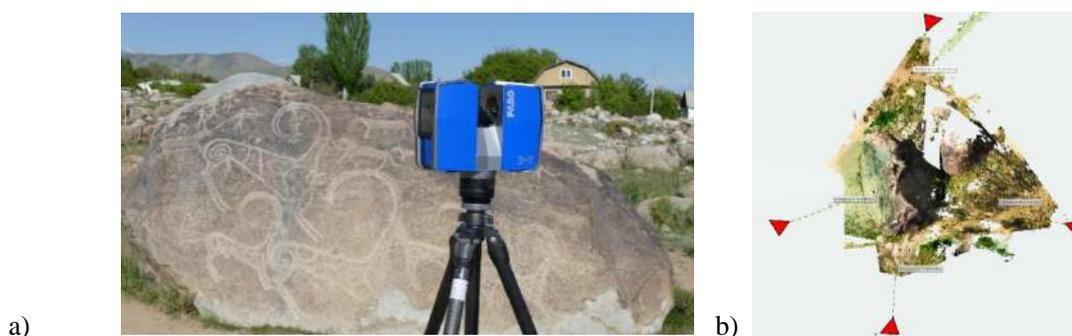
*Fig. 2. Petroglyph scanning using the FARO Focus X330, a) general view, b) scanner positions.*
